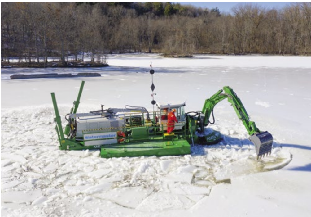
Watermaster, the Canal Corporation's new amphibious multipurpose dredger, undergoes testing on the Mohawk River.
