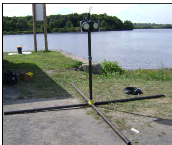
APPENDIX FIGURE G-2.—Steel pipe mount with attached 500-kHz Argonaut-SL acoustic Doppler current profiler used to continuously measure river flow.
