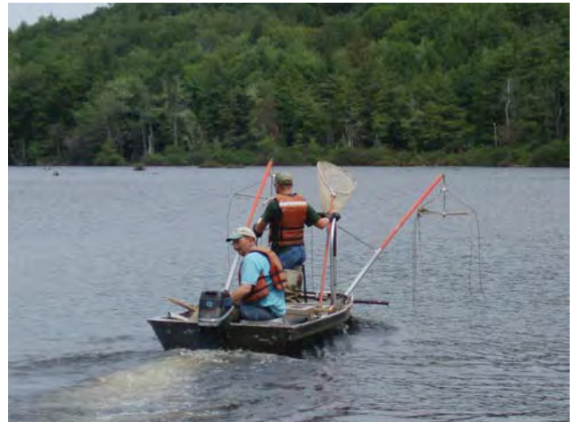
Electrofishing boats are often used as a non-lethal method to sample fish populations.
